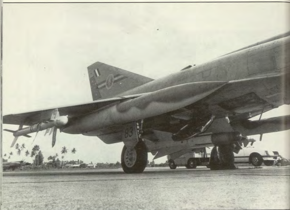
First RAAF Mirage to be loaded with Matra "Magic" Missile. Standard Matra Missile fitted under centre fuselage.
